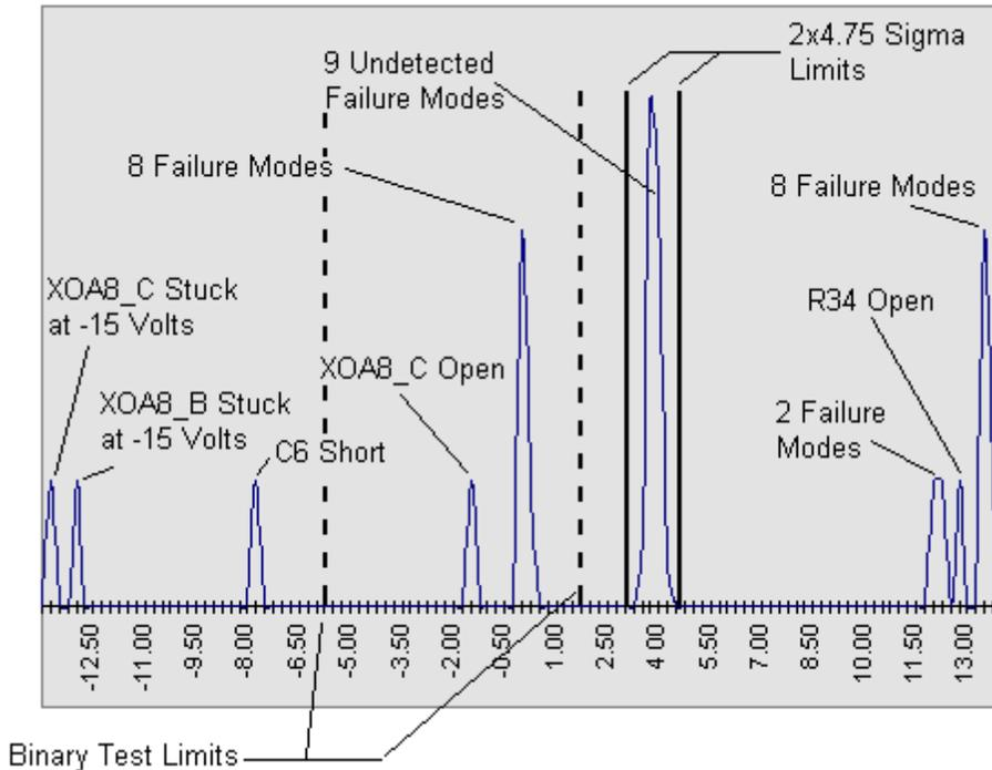
**Figure 4 - Binary test Pass/Fail limits set for specific fault detection characteristics.**
