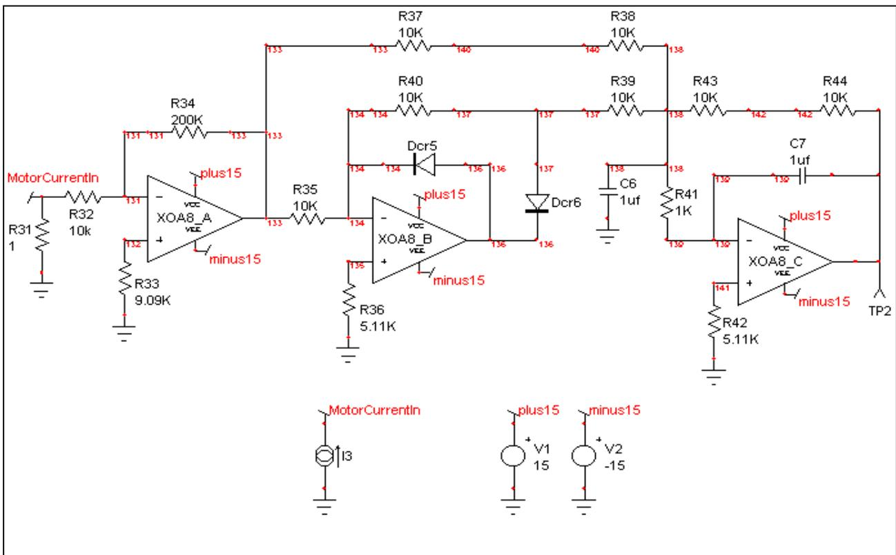
Figure 1 - Motor Current Transducer Input Circuit
